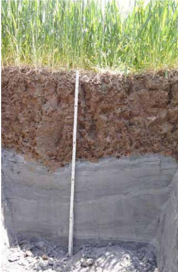
Abb. 2: Soil profile exhibiting the deposited mineral soil above fly ash
