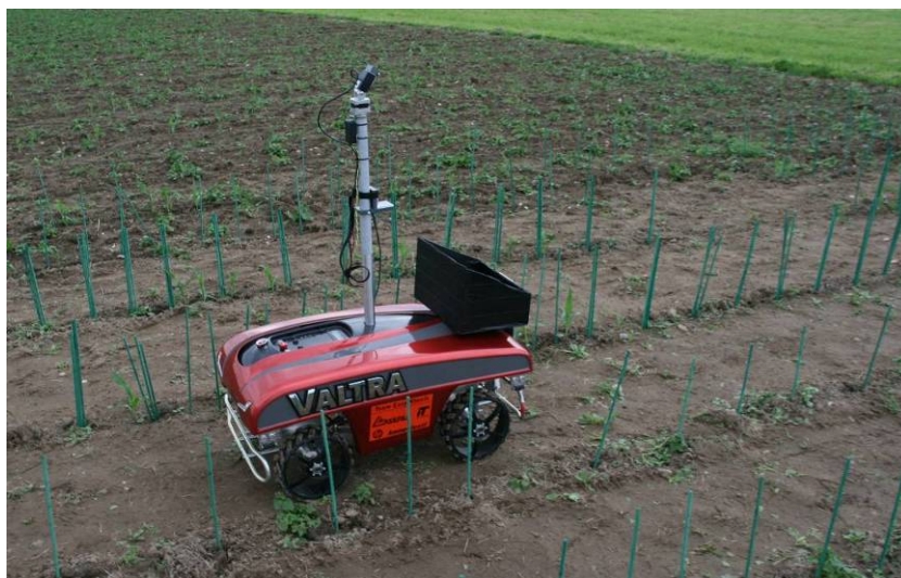
Figure 22: EasyWheels 2010 with a black hopper in Field Robot Event test field.
