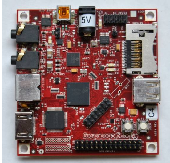
Fig. 5: The BeagleBoard – an embedded computer build around OMAP3530 processor.
