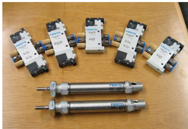
Figure 30: Pneumatic valves and suspension absorbers from one of our sponsors FESTO
