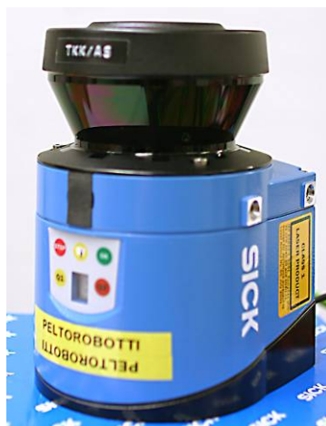
Figure 45: Sick LMS100-1000 laser scanner
