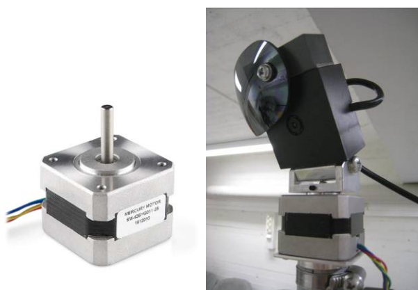
Figure 11: On the left: the stepper motor. On the right: the camera head with re-encapsulated Logitech 5000 with a sun glass.
