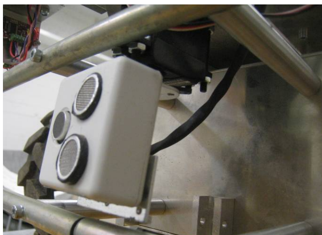
Figure 17: SRF08 and SRF235 installed in front of robot with servo head.
