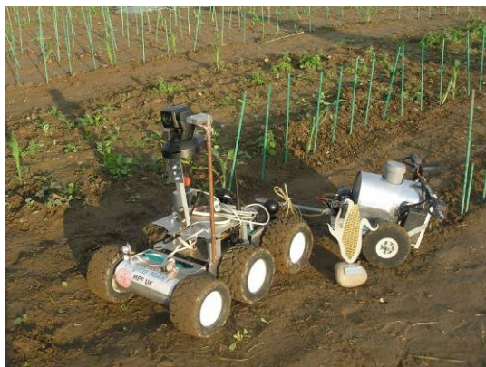
Figure 7: UTrooper platform from Wifobot with a weed extinction device attached.
