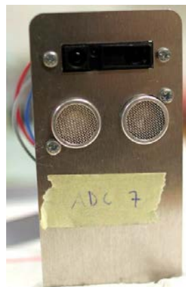
Figure 44: Ultrasonic and infrared module (upside-down)
