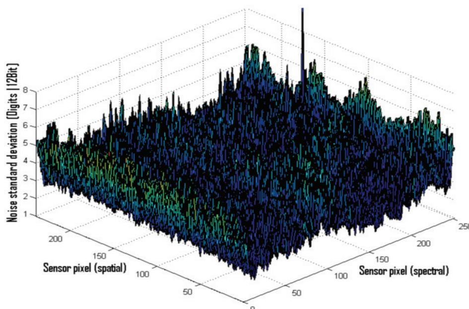
Figure 10: Standard deviation of pixel noise (sample rate 150 fs<sup>-1</sup>, signal intensity average 50 % of 12 Bit)
