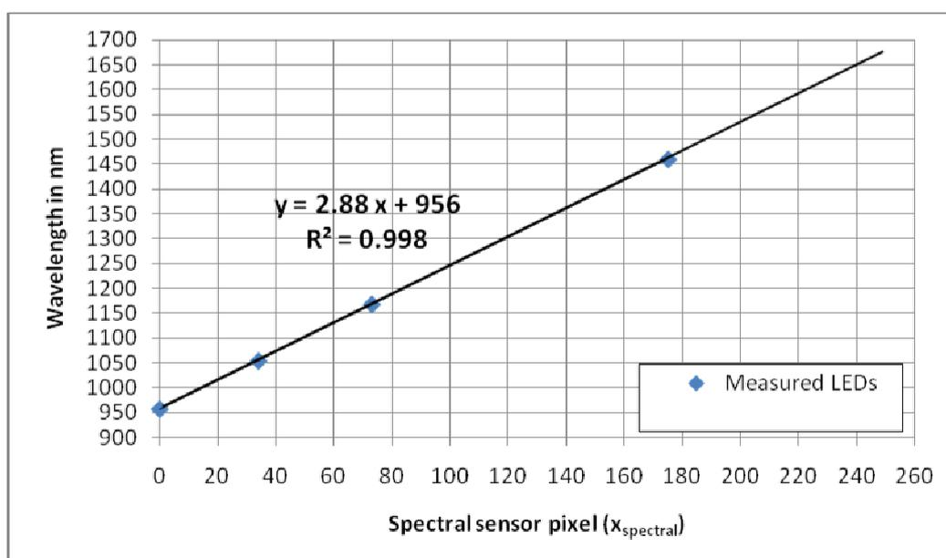
Figure 7: Wavelength/Sensor pixel calibration function of the Helios Core System
