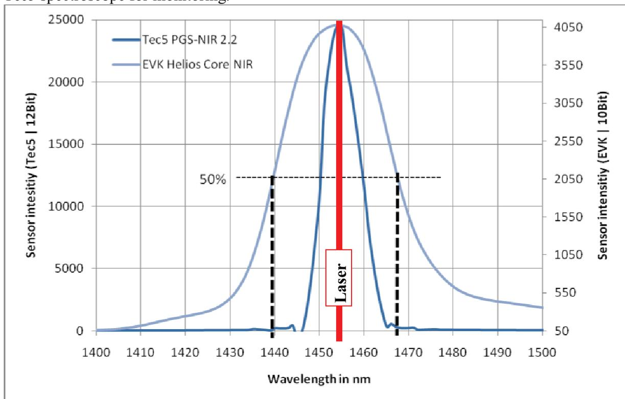
Figure 8: measurement of the spectral resolution of the Helios Core system by scanning the spectral illumination-width of a Laserdiode (Laser-peak at 1454 nm)
