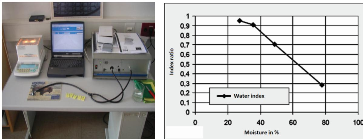
Figure 6: Setup for sponge moisture measuring (left); measured correlation of basic water index / moisture (right)
