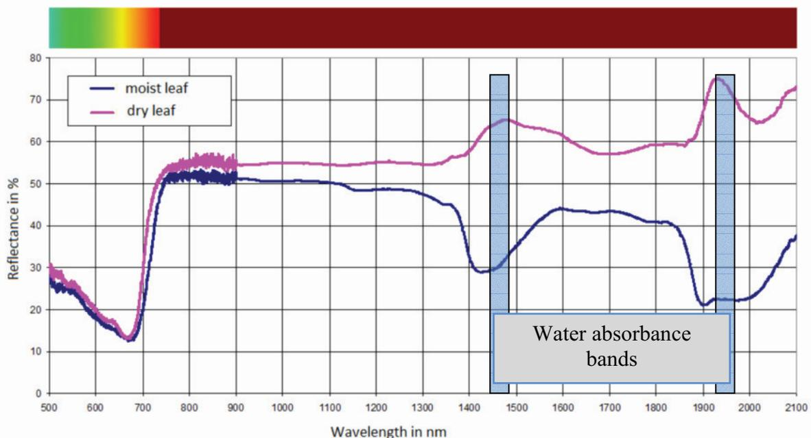
Figure 4: Typical reflectance of a moist and dried leaf with marked water absorption band in the near-infrared waveband
