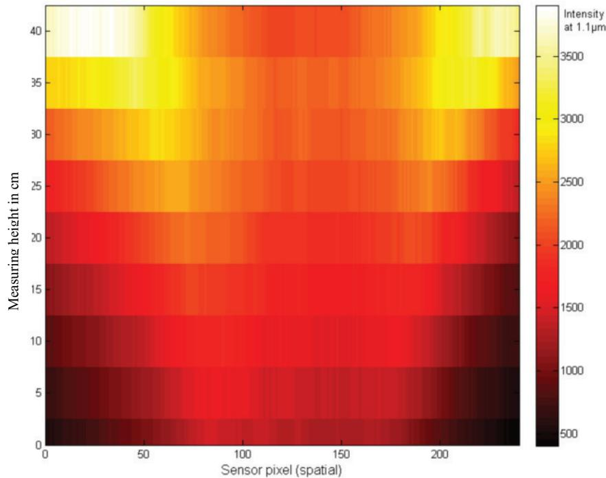
Figure 11: Reflectance intensity of a standardized object in dependence of the object height above system ground level and its spatial location along the scan line (intensity measured at 1.1  $\mu\text{m}$  wavelength, intensity maximum 12 Bit = 4095 Digit)
