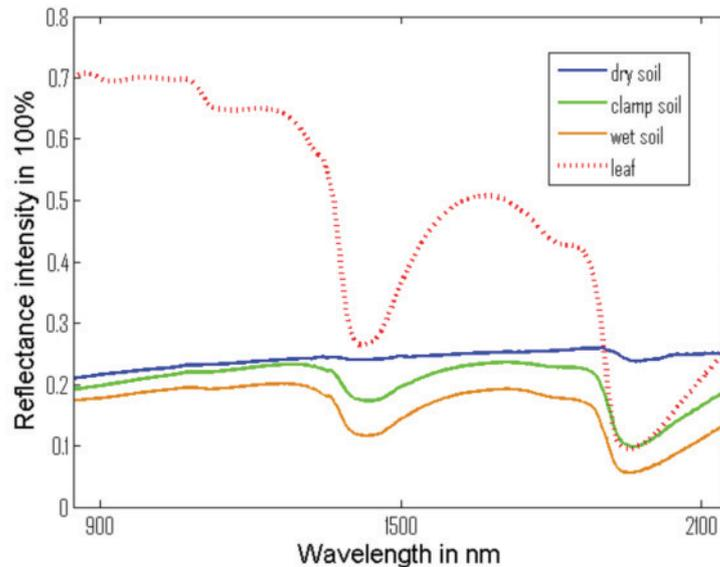
Figure 5: Typical reflectance intensity of soil with different level of humidity
