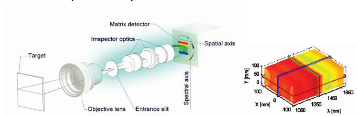
Figure 2: Schematic functional principle of the Spectral imaging sensor system (left) [source: specim.fi]; hyper spectral data cube (right) [source: EVK.biz]
