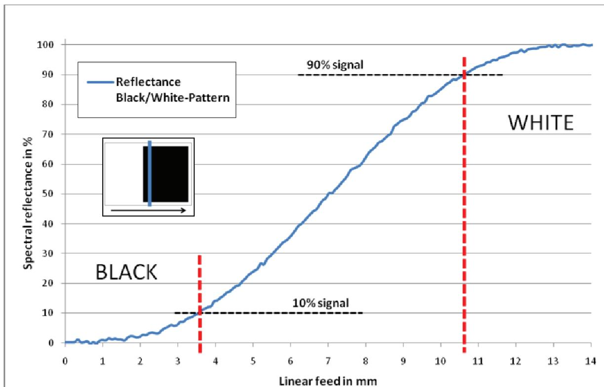
Figure 9: Gradient of reflectance intensity of a single sensor pixel passing a black to white step orthogonal to the scan line (object on system ground level)
