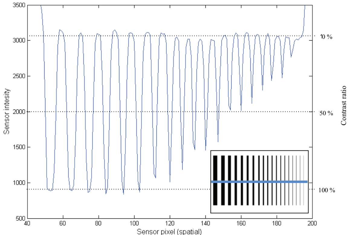
Figure 12: Measurement of the spatial resolution by analyzing the maximum contrast ratio of black lines on white ground (reflectance wavelength of 1.1  $\mu\text{m}$ ; line thickness from 12.5 mm down to 0.6 mm)
