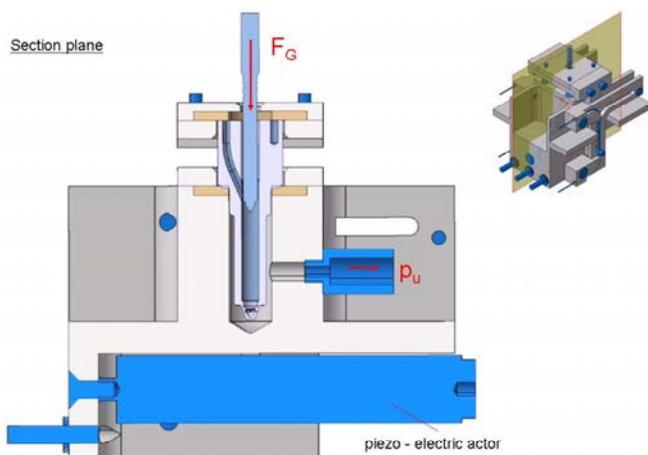
Fig 7: Section plane of the work piece holder with vacuum connection
