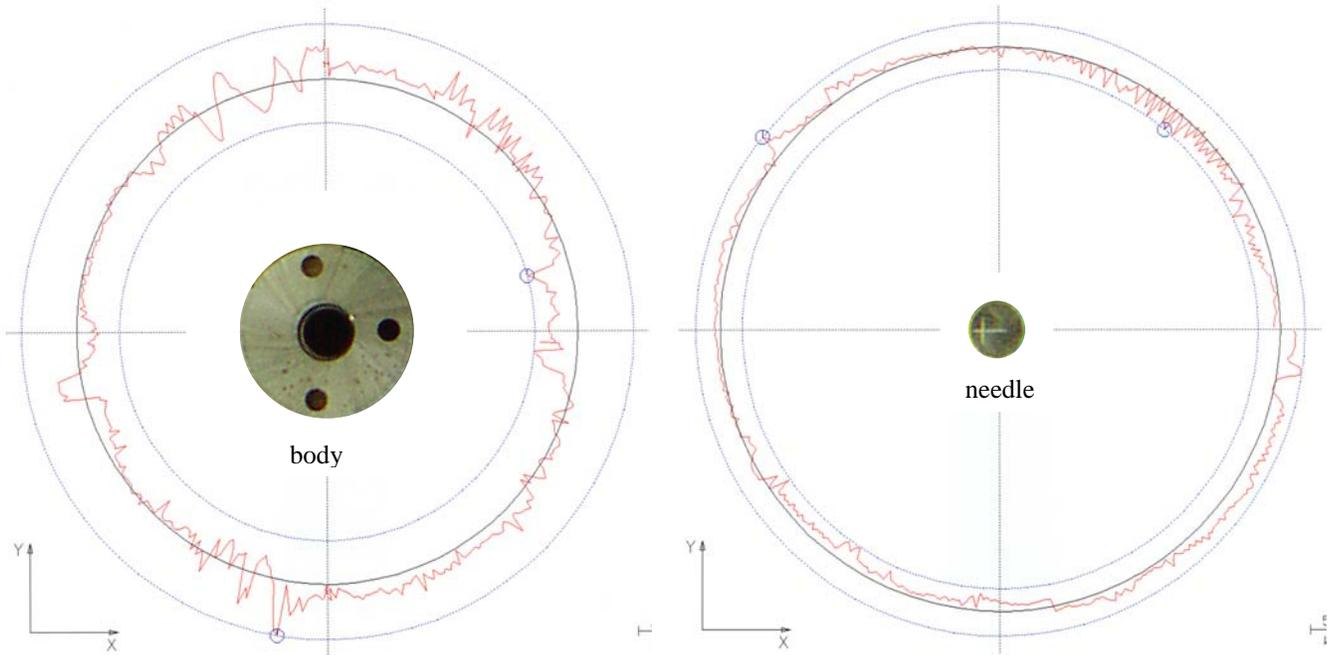
Fig 6: Hole type nozzle - deviation of roundness
