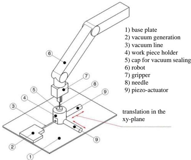
Fig. 2: Principle structure of the assembly device
