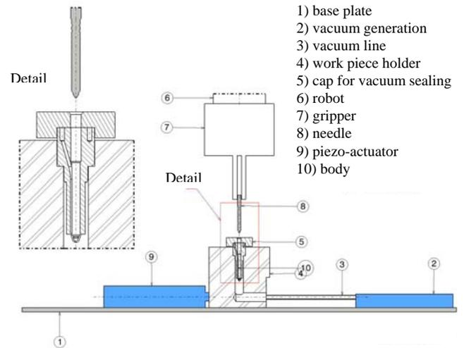
Fig. 3: Cross-section view of the assembly device
