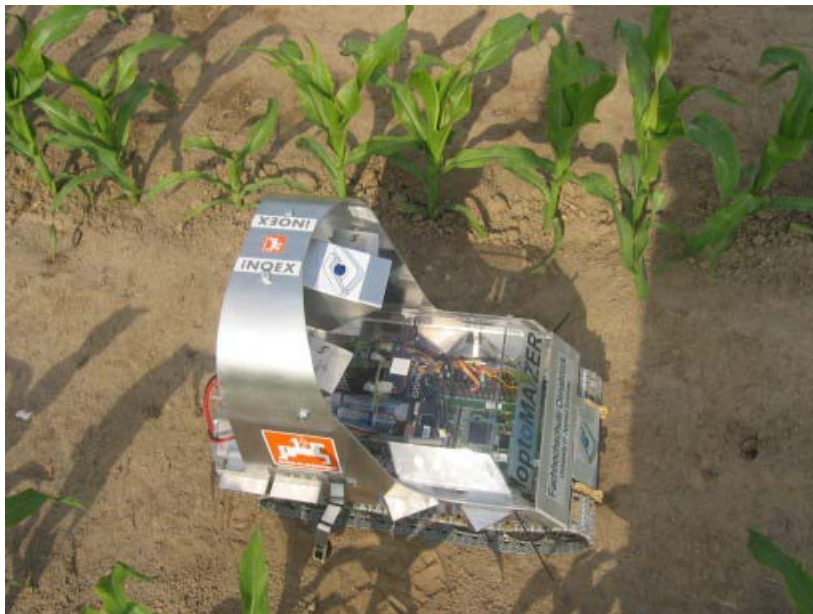
Figure 1: Autonomous field robot optoMAIZER, designed for the Field Robot Event for navigation and counting purposes (Klose 2005).
