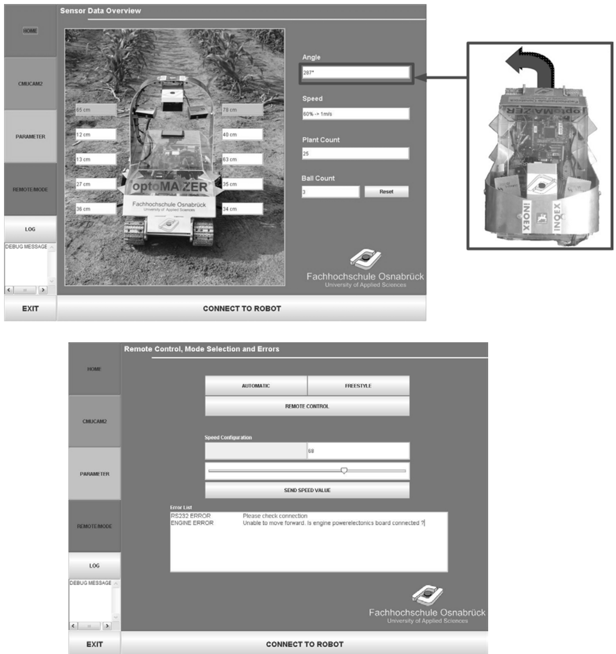
Figure 4: Examples of the graphical user interface for remote services: information of an angle sensor (top), mode selection and error information (bottom).
