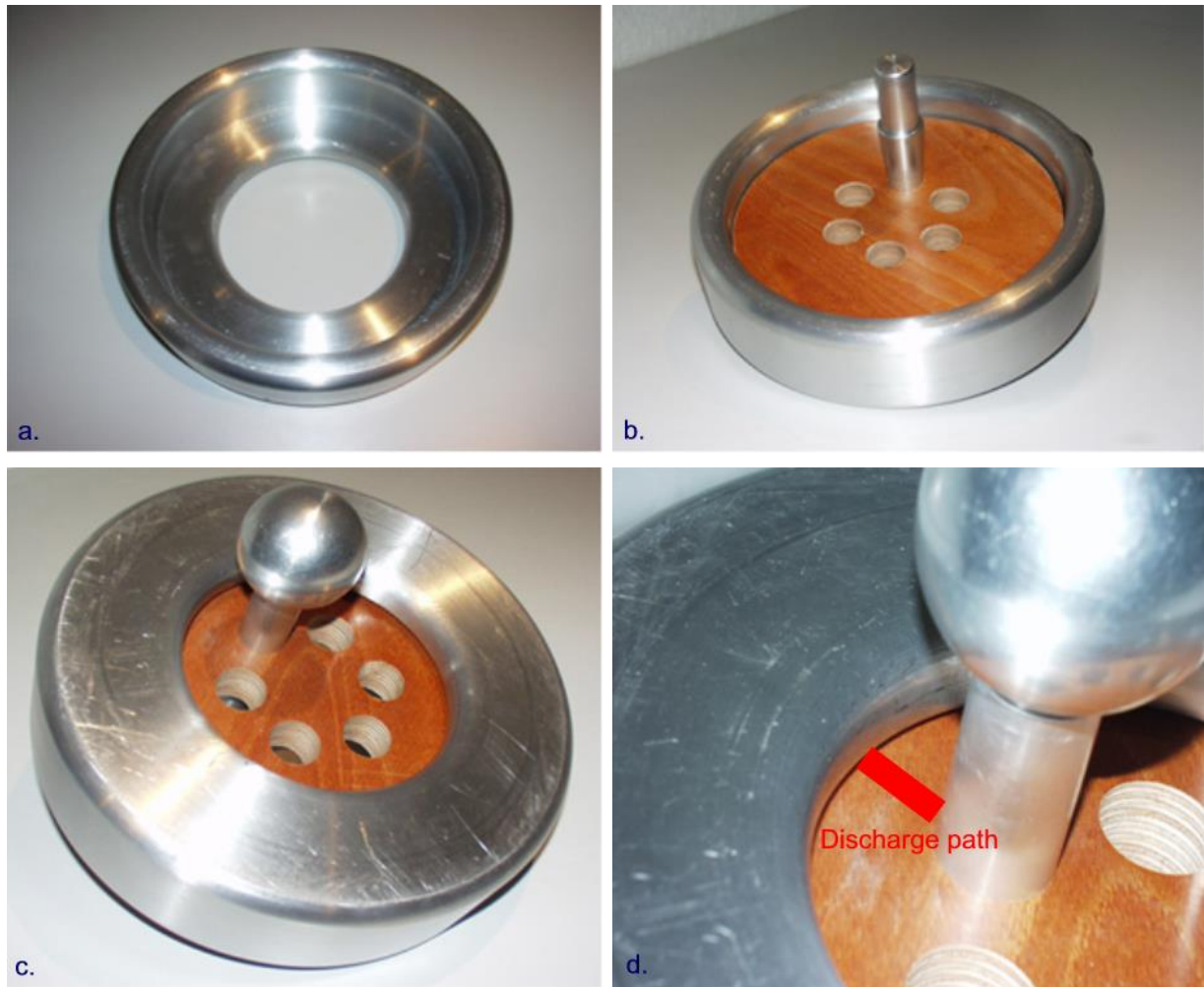
Figure 2 Electrodes and test piece. a. Earthed electrode. b. Top view of earthed electrode with inserted test piece and the high tension electrode in one of the holes in the test piece. c. Bottom view of the earthed electrode with inserted test piece and the high tension electrode in one of the holes in the test piece. d. Magnified view of Figure c. with discharge path marked.
