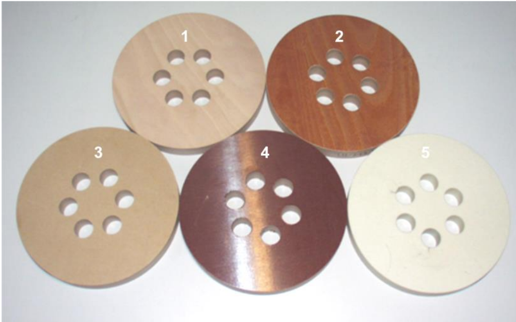
Figure 3 Tested types of material. 1. LDW, sanded with grade 60 paper. 2. LDW, platen finish. 3. LDW/PB without surface treatment. 4. LDW/PB with surface treatment. 5. Durostone
