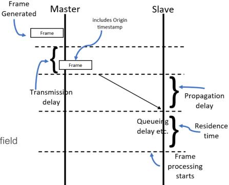
$T_{slave} = T_{Origin} + P_{delay} + T_{residence} + T_{transmission}$
