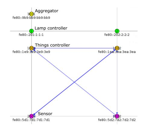
10 Street lamps each with 1 sensor placed with 25 m distance from each other
