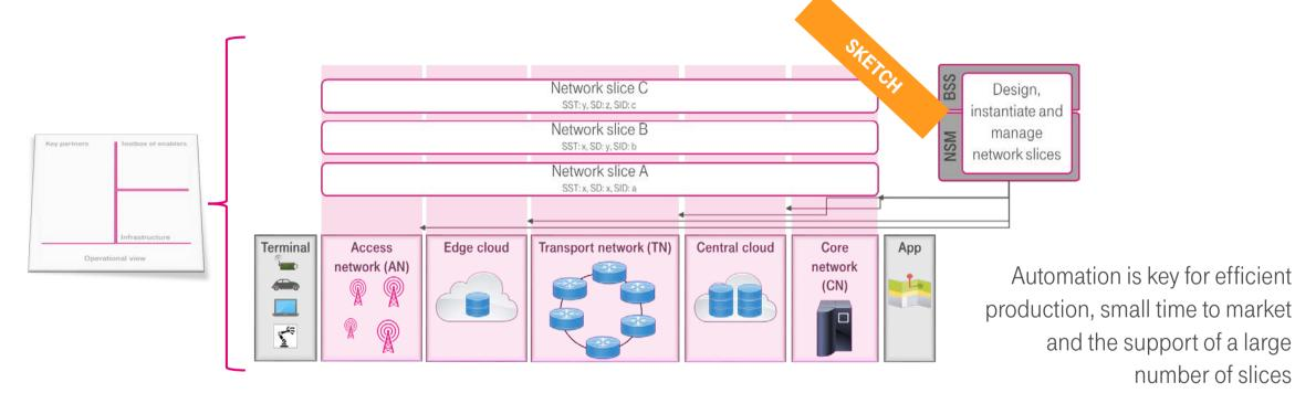
Network slicing needs to consider the whole E2E chain and each network slice subnet needs to support network slicing - waiting for 3GPP Rel. 16+ is not enough.
