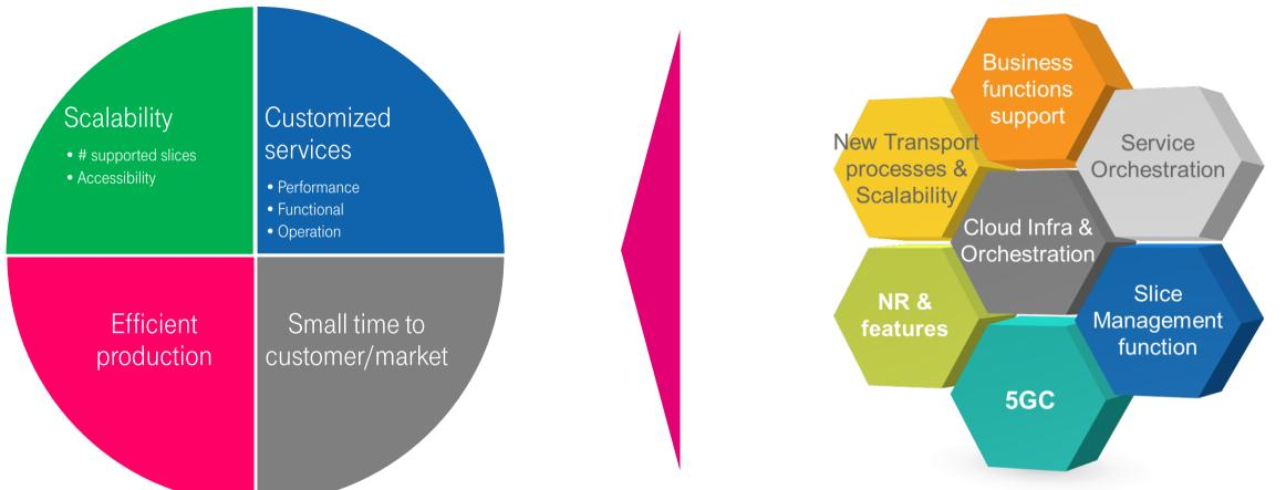
Network slicing: Provisioning of customized services in a scalable and efficient way with small time to customer/market.
