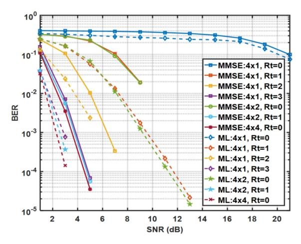
Multi user MIMO-OFDM systems' performance comparison in terms of BER with proposed scheme, while using MMSE detector and ML detector
