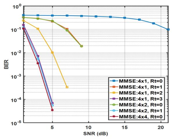
Multi user MIMO-OFDM systems' performance in terms of BER with proposed scheme, using MMSE detector.
