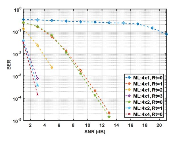
Multi user MIMO-OFDM systems' performance in terms of BER with proposed scheme, using ML detector.
