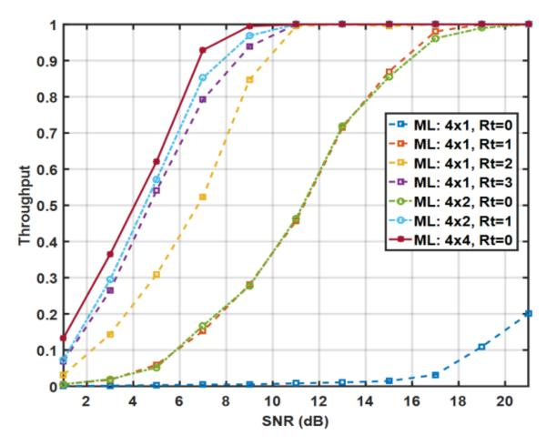
Multi user MIMO OFDM systems' performance in terms of throughput with four transmitter antennas  $N_{Tx}=4$ , using ML detector
