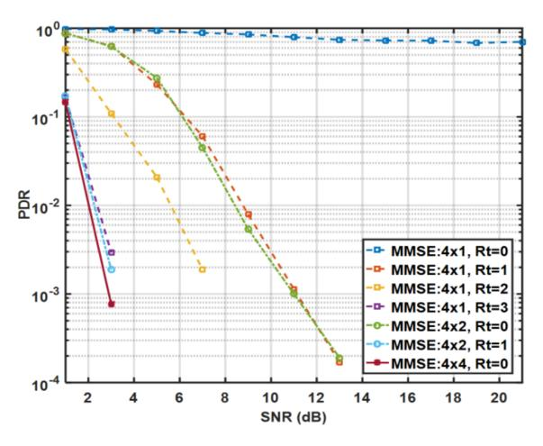
Multi user MIMO OFDM systems' performance in terms of PDR with four transmitter antennas  $N_{Tx}=4$ , using MMSE detector
