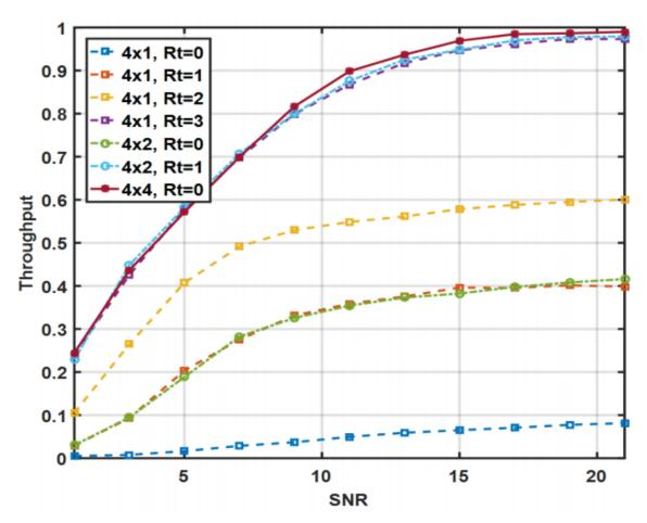
Multi user MIMO OFDM systems' performance in terms of throughput with four transmitter antennas  $N_{Tx}=4$ , using MMSE detector
