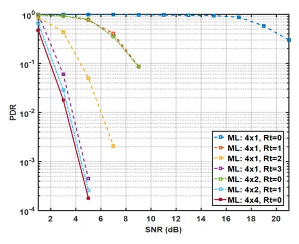
Multi user MIMO OFDM systems' performance in terms of PDR with four transmitter antennas  $N_{Tx}=4$ , using ML detector
