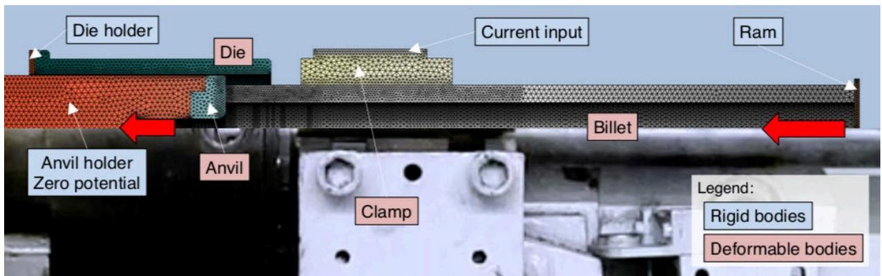
Figure 4. Outline of the FEM model in contraposition to the real system.
