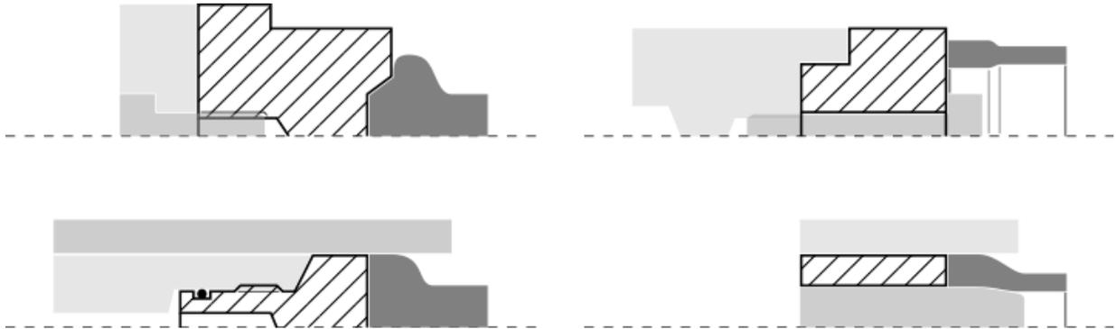
**Figure 8.** Some anvil designs (dashed) proposed to tackle specific requirements
