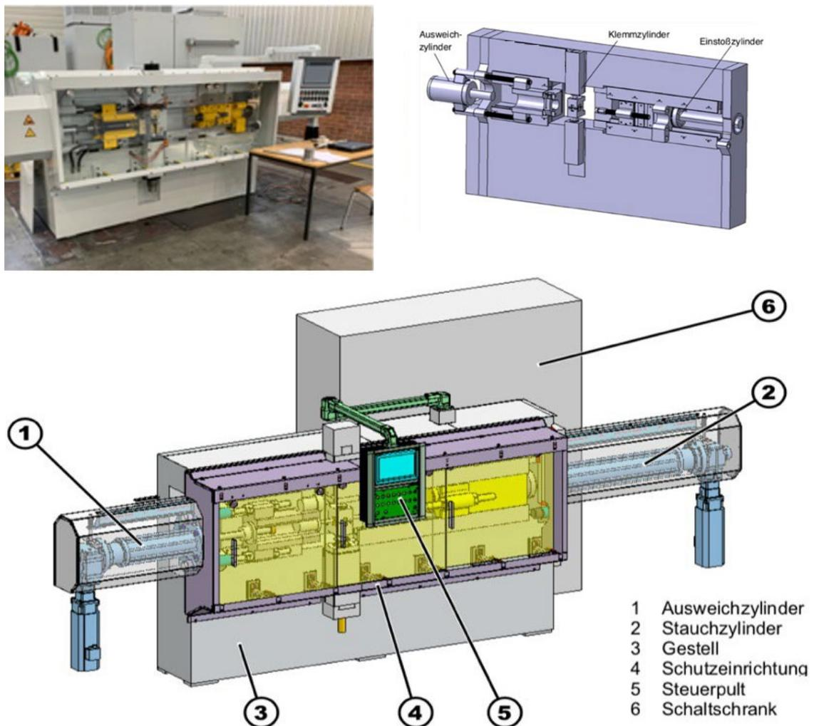
**Figure 5.** modification of the machine with state-of-the-art direct-drive servo motors and new control system with developed control strategies. Top: final machine (left) and schematic CAD of the original hydraulic machine (right). Bottom: CAD with the implemented systems.
