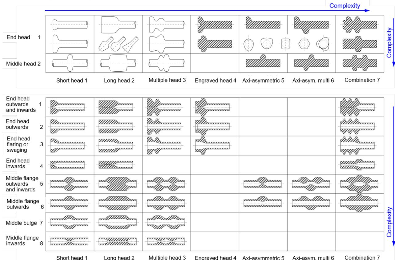
Figure 2. Classification chart for electroforging products
