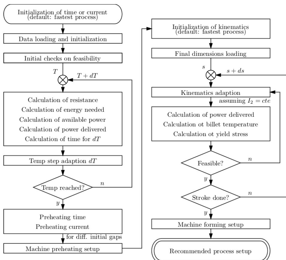
Figure 3. Overview of the proposed analytical model for the prediction of process parameters in electroforging
