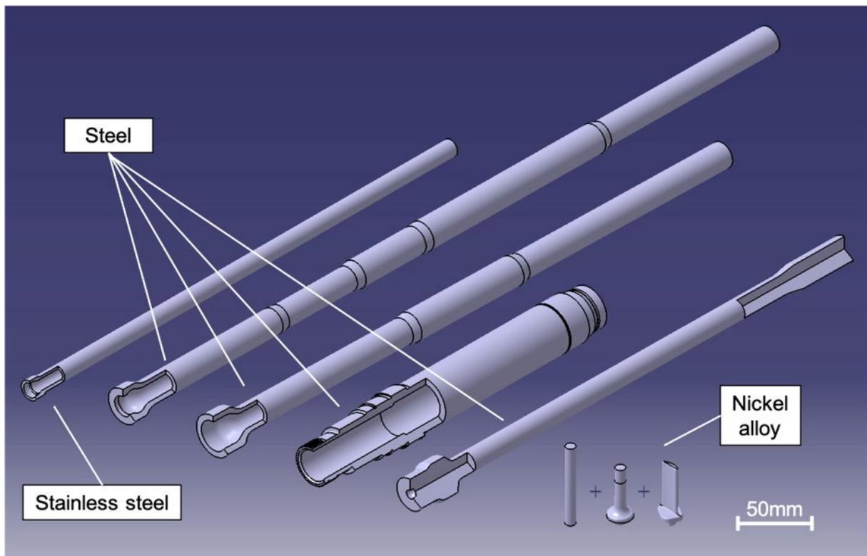
**Figure 1.** Component prototypes covering the spectrum of geometries objects analyzed in the research project: 4 tubulars and 2 solid industrial parts.
