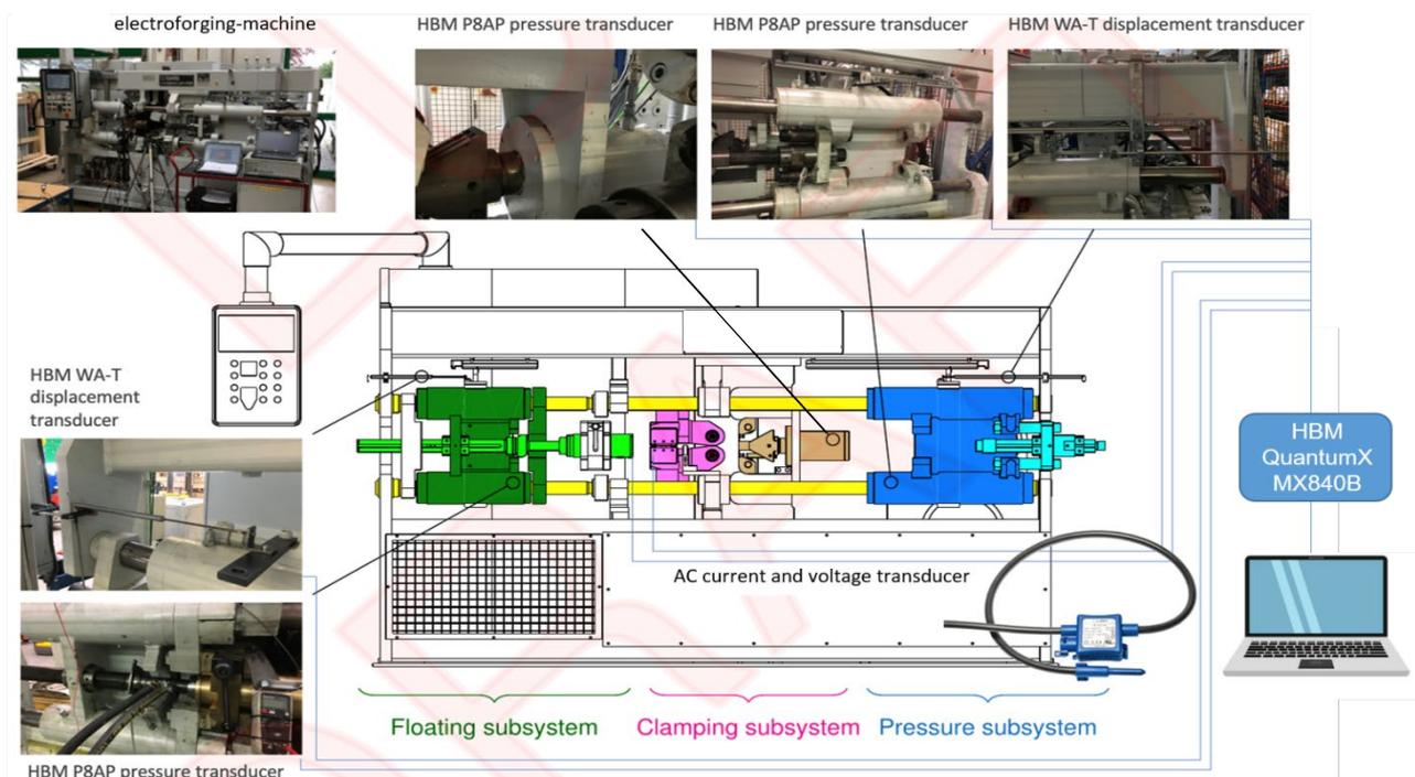
**Figure 9.** Outline of the DAQ designed for the systematic data acquisition of electroforming experimental tests in the electric upsetter.
