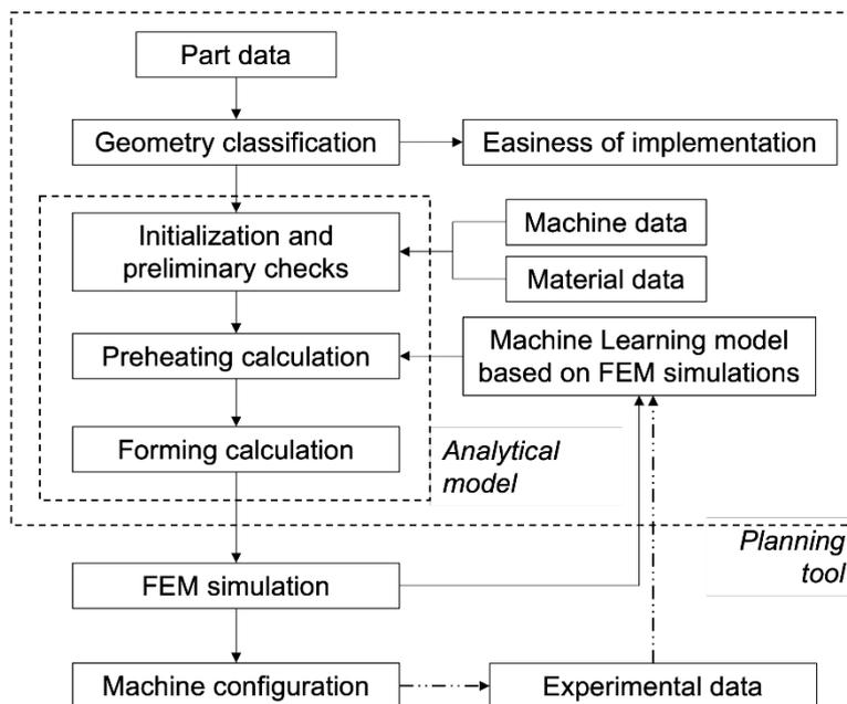
Figure 6. Schema of the planning methodology for electroforging, based on analytical and numerical models.
