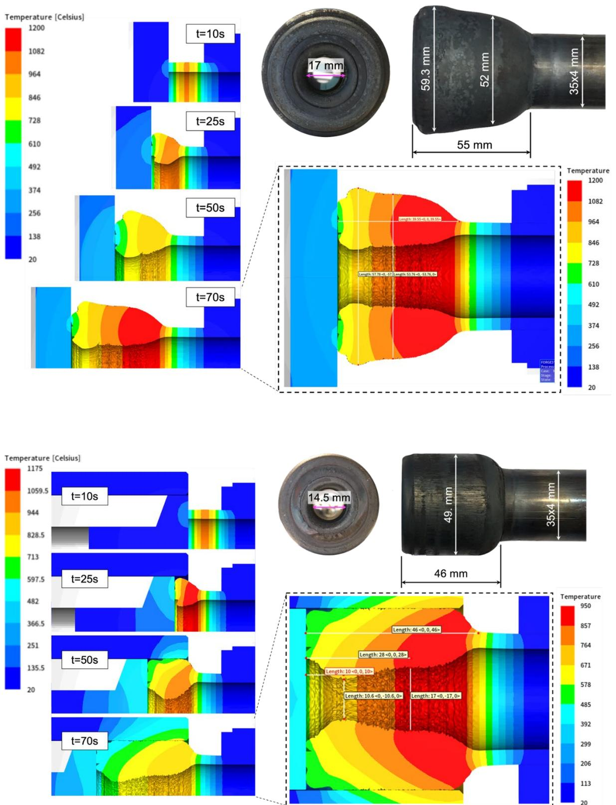
Figure 10. Process configuration using the methodology developed during the project for the free electroforming and closed die electroforming of a tube (geometry type TE22) for a vehicle anti-roll component of low carbon steel. Process evolution is shown in the left, with comparison of final geometry between simulation and forging on the right.
